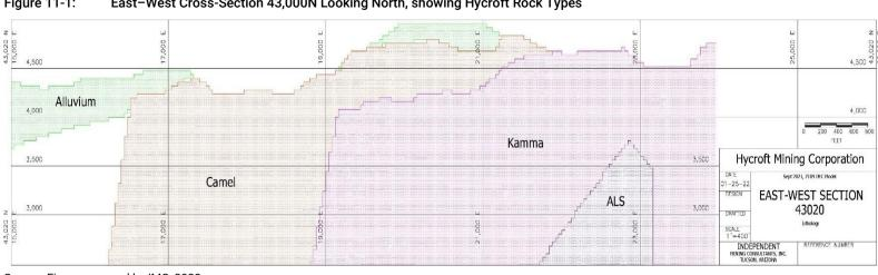
Figure 11-1: East-West Cross-Section 43,000N Looking North, showing Hycroft Rock Types
