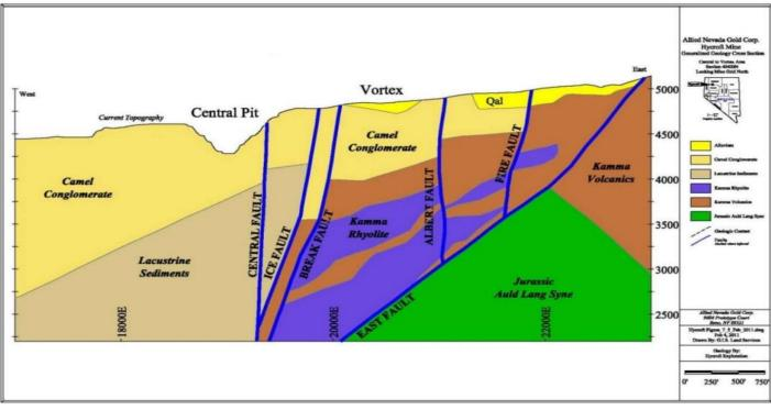
Figure 6-4: Vortex to Camel Hill Generalized Section
