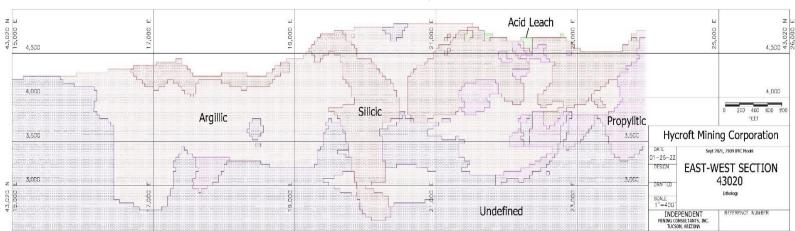
East-West Cross-Section 43,000N Looking North, showing Hycroft Alterations Figure 11-2:
