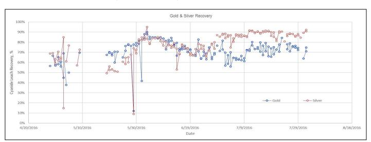
Figure 10-4: Demonstration Plant Cyanide Leach Recovery of Au and Ag
