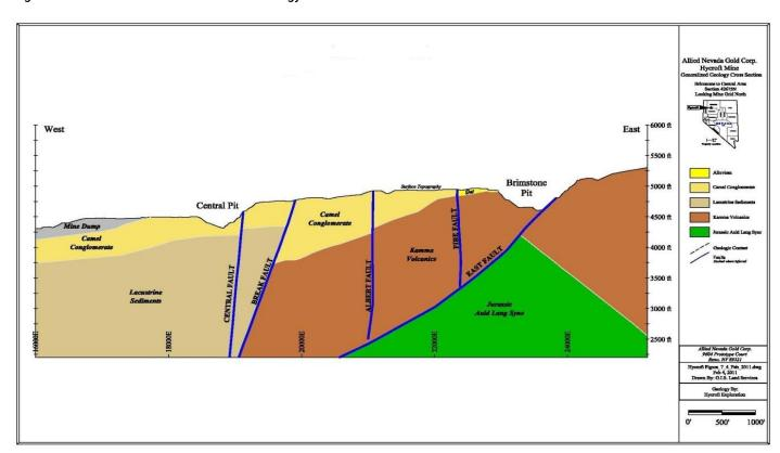
Figure 6-3: Brimstone Generalized Geology Cross-Section
